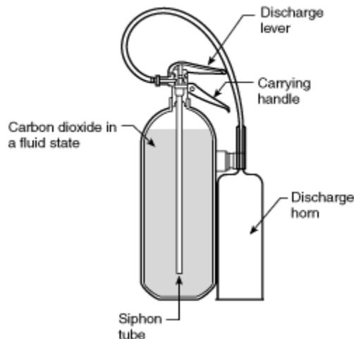
**Figure D-4.3(b) Carbon dioxide extinguisher.**
