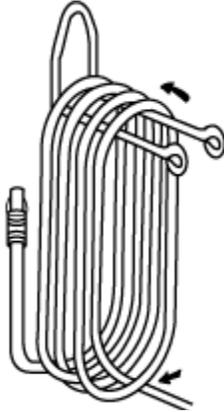
(d) Adjust coil so that nozzle is in the downward position as shown in Figure A-4-3.2(d). (Hose coiled in this manner will pull off free of twists).
