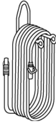
(e) Place nozzle in holder with handle forward in the closed position. [See Figure A-4-3.2(e).]
