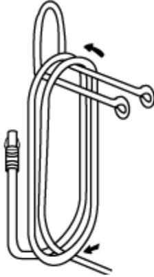
(c) Repeat Steps (a) and (b) until all hose is coiled on support. [See Figure A-4-3.2(c).]
