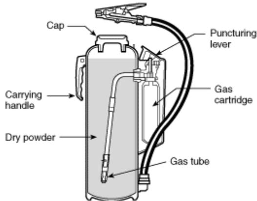
**Figure D-4.6.1(b) Stored-pressure dry powder extinguisher with wand applicator.**
